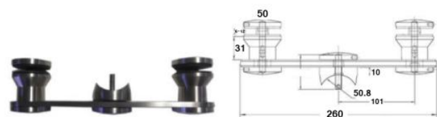
GLH1010K-50-50.8 Double Glass Retainer (50 x 50mm) 316
