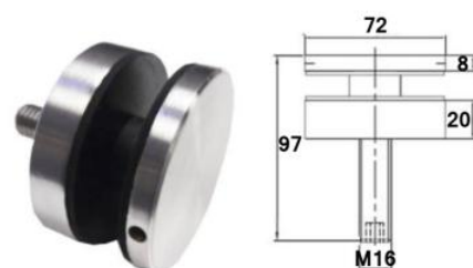
JK-1016 Solid Threaded Body – Flat Head M16 Removable Thread 304/316
