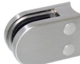
KLH13.52-15MM-48.3-SATIN 316 Grade Satin Finish Suitable for 13.52 and 15mm Glass
